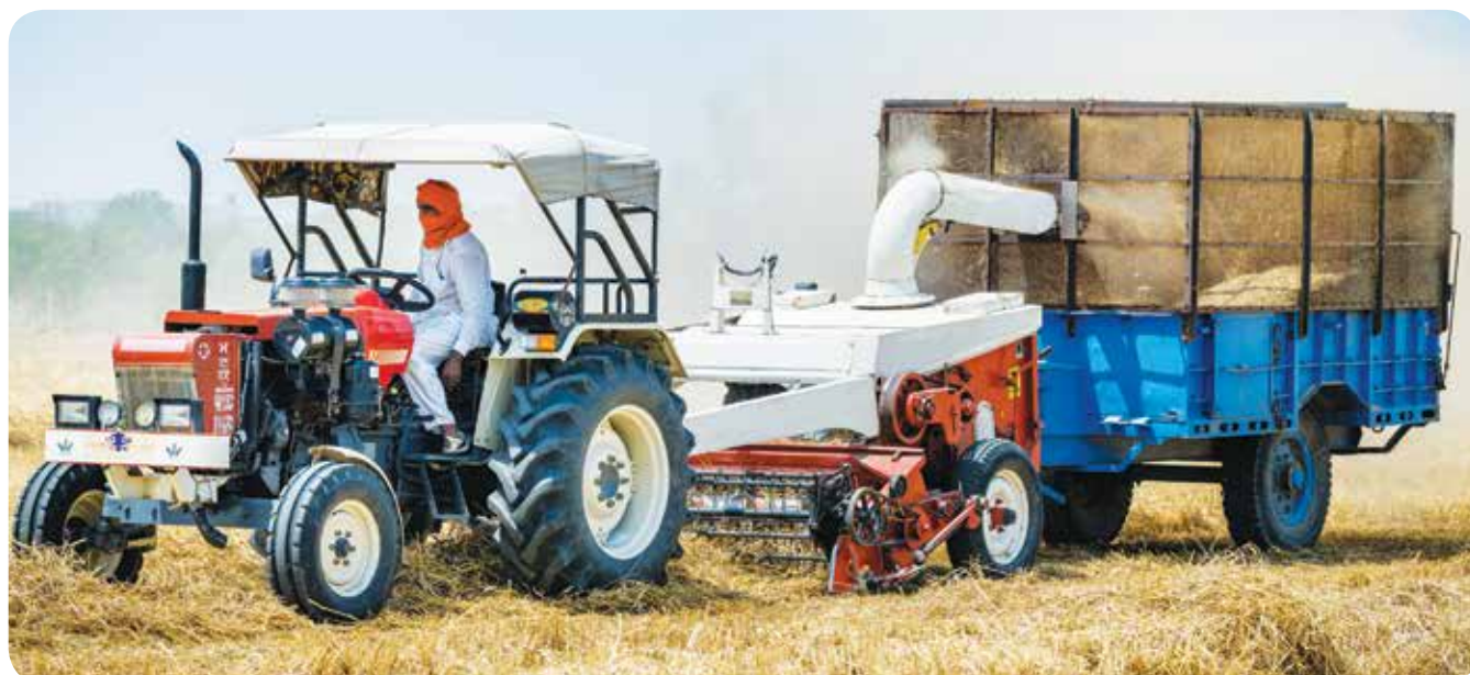
Straw picking, chopping and loading machine used in combine harvested area
