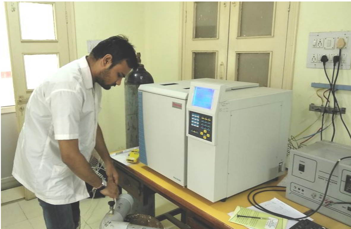
Photo 4: Analysis of breath samples in GC
